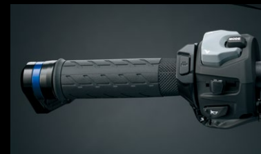
Grip Heater 57100-25810-000 This grip heater has 3 adjustable heat level settings. You can keep the entire surface of the grip warm for comfortable riding.
