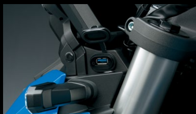
USB Socket 39100-25810-000 A socket to help charge electronic devices through USB connection. There is a cover lid in order to protect the socket from dust, sand, etc. It is USB Type-A with output of 5V/2A.
